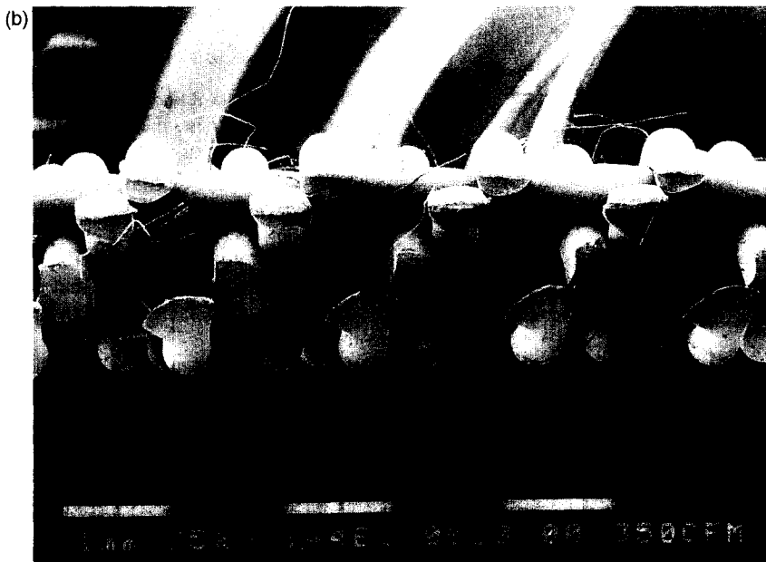
Fig. 2(b). Scanning electron micrograph of a 350 cfm dryer fabric showing edge construction ( \times 14 ).
